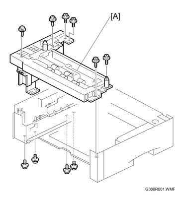
**NOTE:** Before removing the paper feed unit, turn the main unit over and remove all screws indicated with an arrow.
