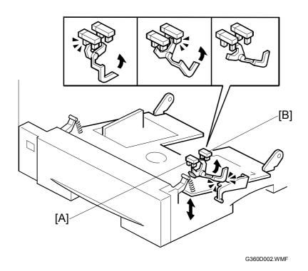
[A]: Remaining paper sensor 1 [B]: Remaining paper sensor 2
