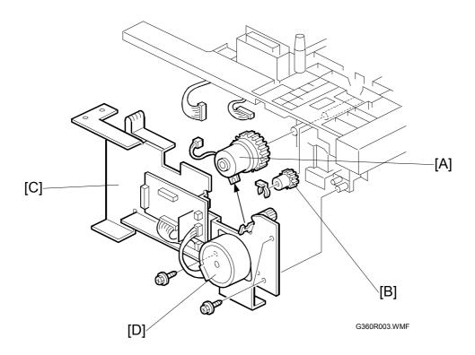
[A]: Paper feed clutch (∜ x 1, 1 gear) [B]: Paper feed gear (∜ x 1) [C]: Motor bracket (♠ x 3, ➡ x 2) [D]: Motor (1 gear, ➡ x 1)
